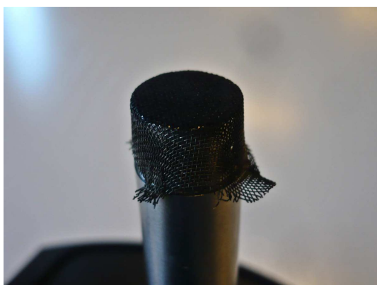
Strainer blocked by soot
